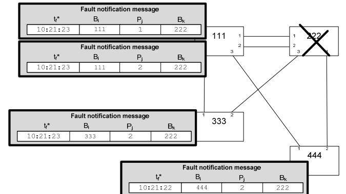
Fig. 8. Bridge fault. Bridge 222 fails, causing the generation four fault notification messages.
