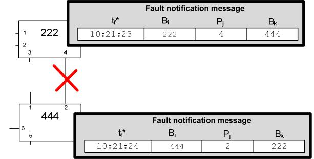
Fig. 7. Link fault. The link between bridge 222 and bridge 444 fails, causing the generation of two fault notification messages.
