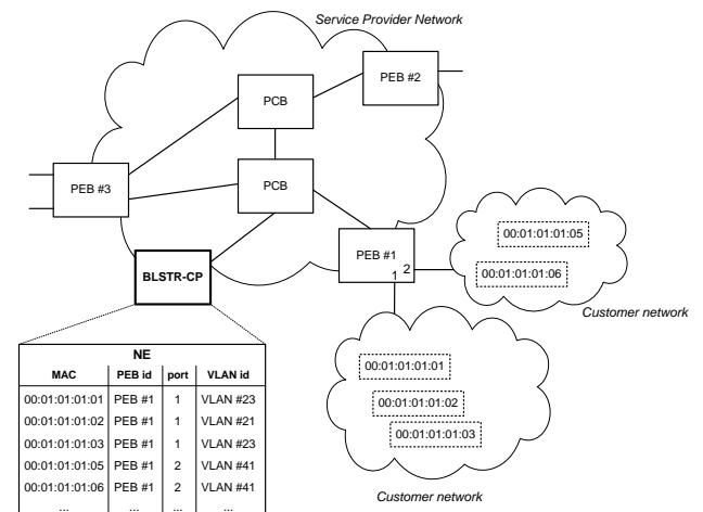
Fig. 3. Network Endpoint table (NE) for a sample Provider Bridges network (PEB: Provider Edge Bridge, PCB: Provider Core Bridge).
