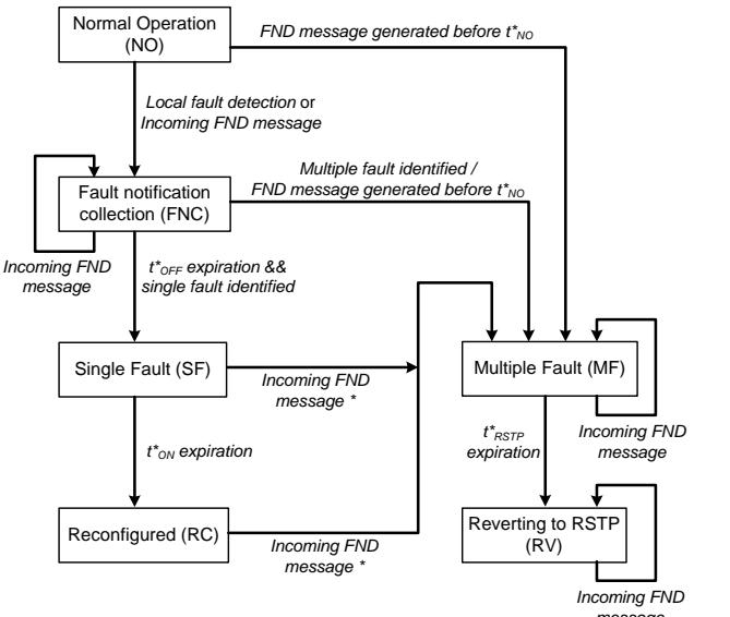
Fig. 5. BLSTR multiple resource fault control strategy (\* A FND message arriving to bridges in *SF* or *RC* denote always a multiple fault).
